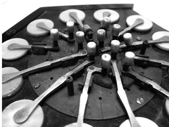
Figure 27. The Pallets, action block and levers of the Chambers Collection Open Pallet concertina, ref. CC1. Photo N.Wayne © The Chambers Collection.
