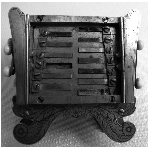
Figure 11. Reed-plate of an early 17-Key Wheatstone Symphonium, c.1825–1829. Photo N.Wayne © The Concertina Museum Collection Collection.
