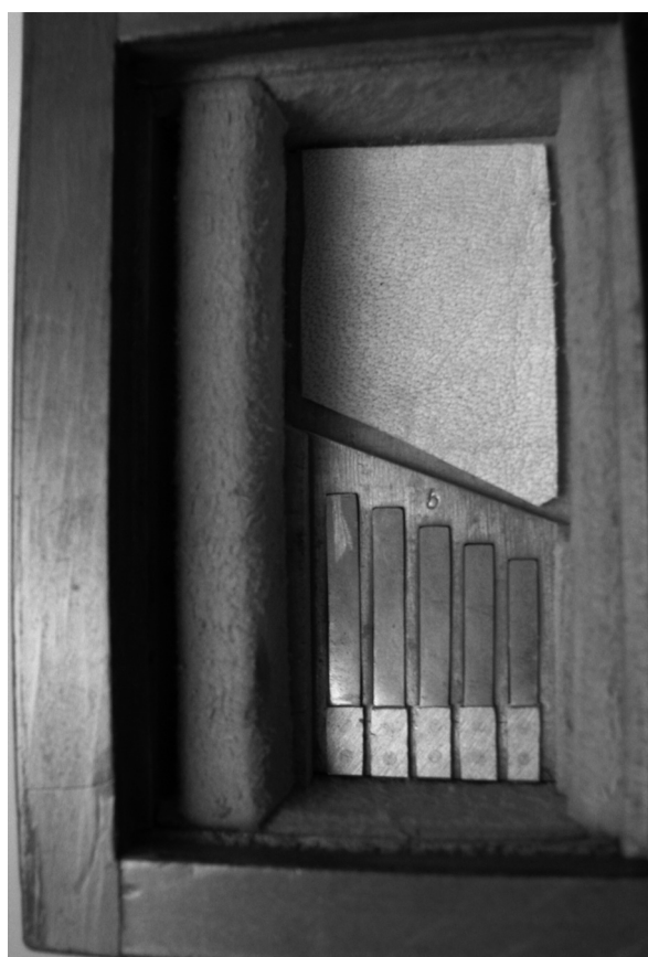
Figure 5. The reed-plates of the 5-key Demian accordion, c.1829. The Horniman Museum, Wayne Collection, cat. no: M15-1996. Photo N.Wayne, © The Horniman Museum.
